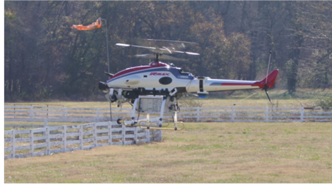
Figure 58: UAV test-bed at Georgia Tech: The base airframe is Yamaha RMAX.
