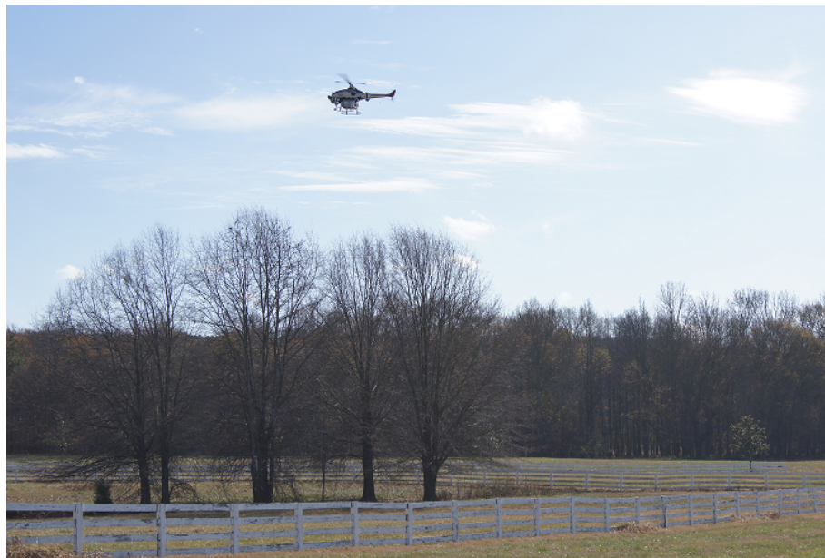
Figure 82: UAV test-bed is avoiding the tree obstacle in the flight test.
